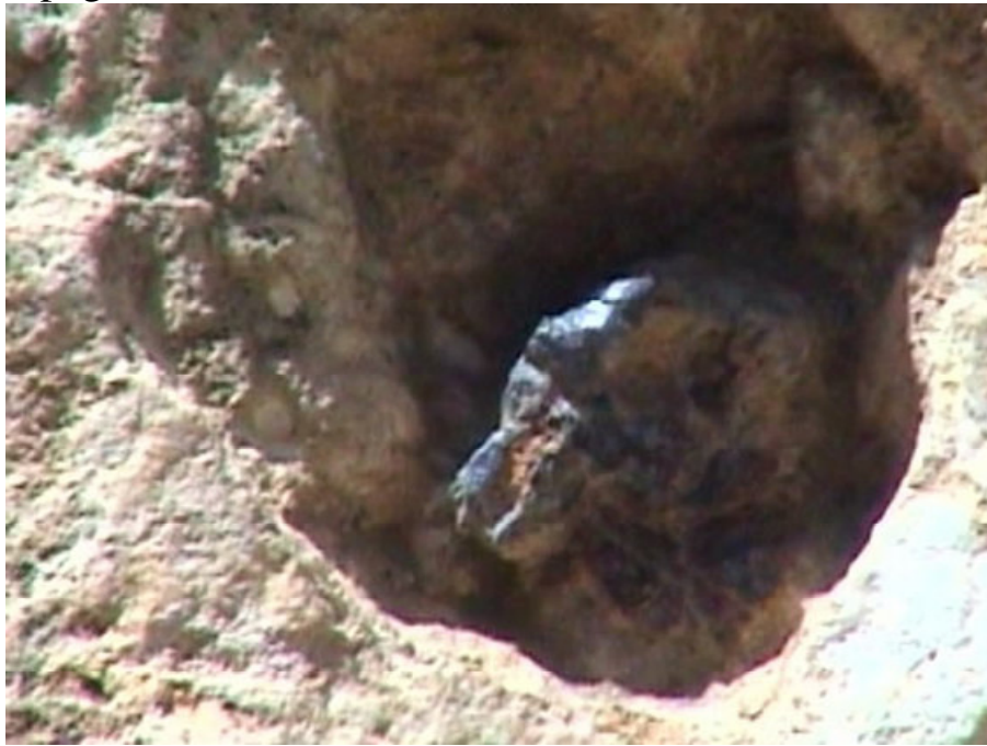
The remains of the metal peg, the outer end of which was sheared off by some tremendous force
